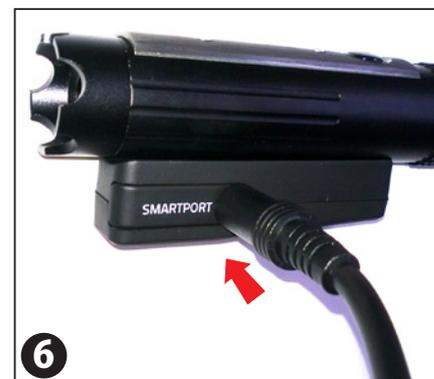
6 <Option 1> Connect the AV cable to the Smartport.
