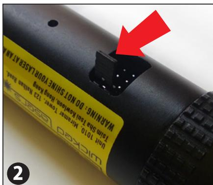
2 Remove the jumper shown here before connecting the Smartport.
