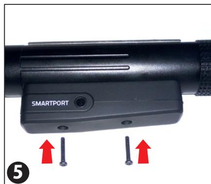
5 Use the two screws to secure the Smartport in place.
