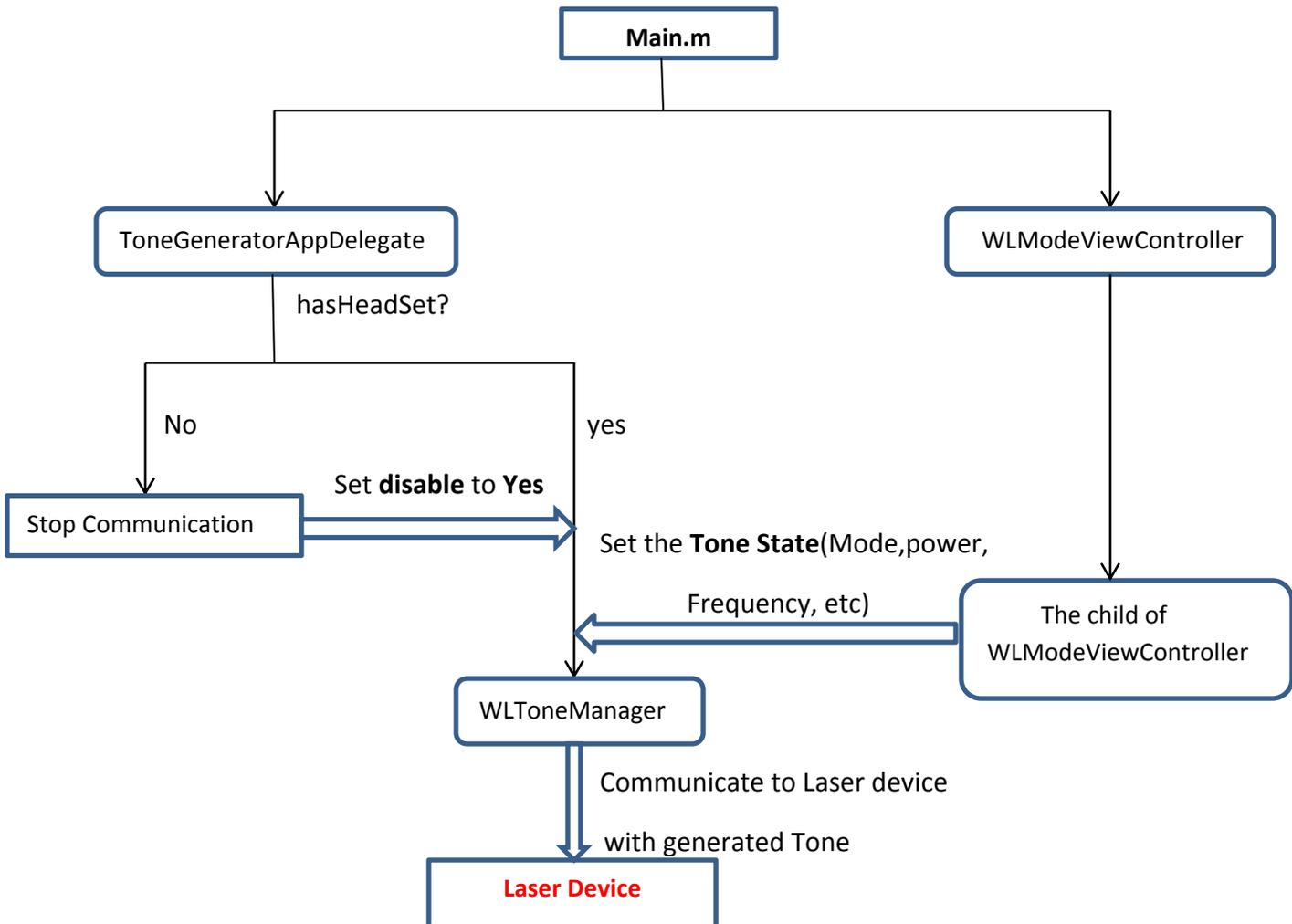
Figure1. Work flow of iOS Evo Laser app
