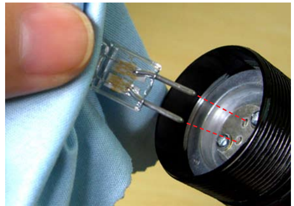
Align 2 prongs with 2 holes to insert replacement bulb.
