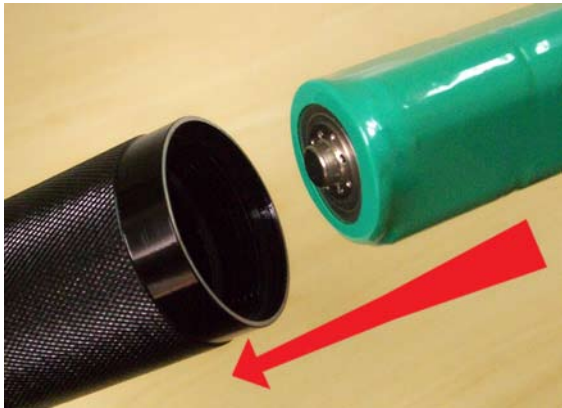
Insert battery positive end first.
