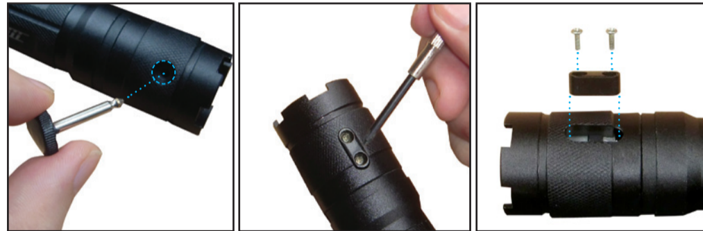
Removing the Safety Interlock from the Endcap will disable the laser.
