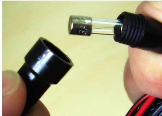
Replace burnt-out fuse.
